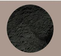
Green Microzest 50 Charcoal is manufactured by processing at very high temperatures coconut shells
